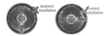
\*\*Annexe A: These wide angle lights must be correctly positioned. Look through the outer lens and you will see lines on the primary optic. The lines in the optic must be vertical, see photos\*\*
