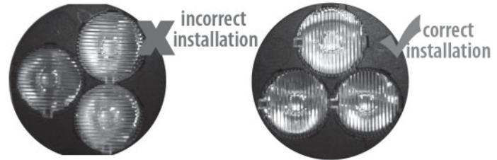
\*\*Annexe A: These wide angle lights must be correctly positioned. Look through the outer lens and you will see lines on the primary optics ie the 3 small lenses. The lines in the optic must be vertical, see photos\*\*
